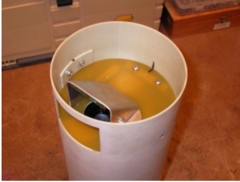
Details of the mirror holder and window assemblies.
