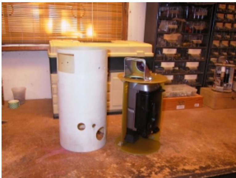
The Samsung 8mm camcorder mounted in the carrier. The white tube slides over the carrier and adds strength to the payload section, which is weakened by the large window hole.
