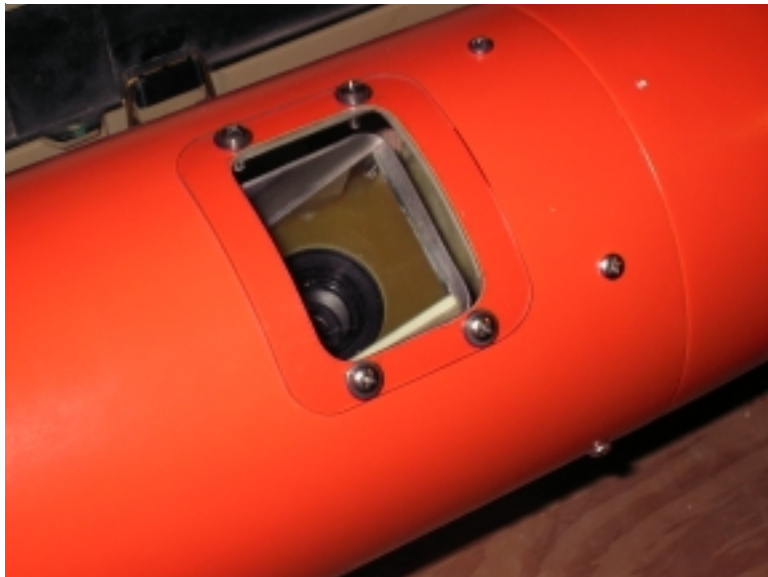
Details of the mirror holder and window assemblies.
